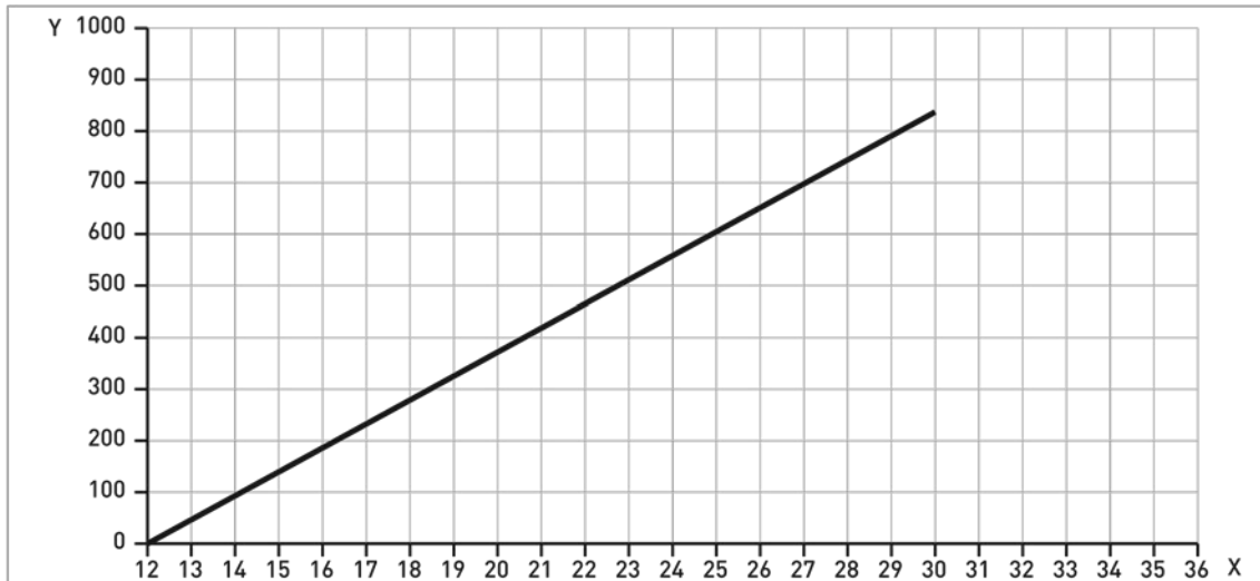
Figure 5: Minimum power supply voltage for an output of 21.5 mA at the terminals (Non-Ex and Hazardous Location approval (Ex i / IS))
