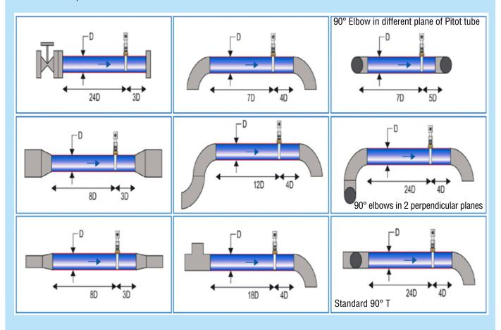
Chosen location for 5RD Pitot tube series set up in piping systems really matters because of the turbulence (secondary flow) in the flow created by the pipe configuration which can compromise the measurement accuracy. If the 5RD Pitot tube series is set up on shorter distance than advised, accuracy might be compromise but measurement repeatability will remain exact.
